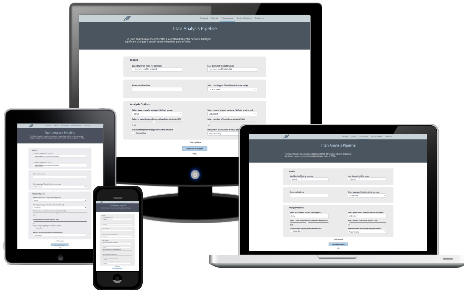
Figure 2: The Web Server Layout Dynamically Adapts to Different Devices. From left to right, the Figure shows the layout of the input-page on a tablet, mobile phone, desktop and laptop. The inputs align horizontally on the desktop and laptop, and vertically on the phone and tablet. Produced by A.T.
